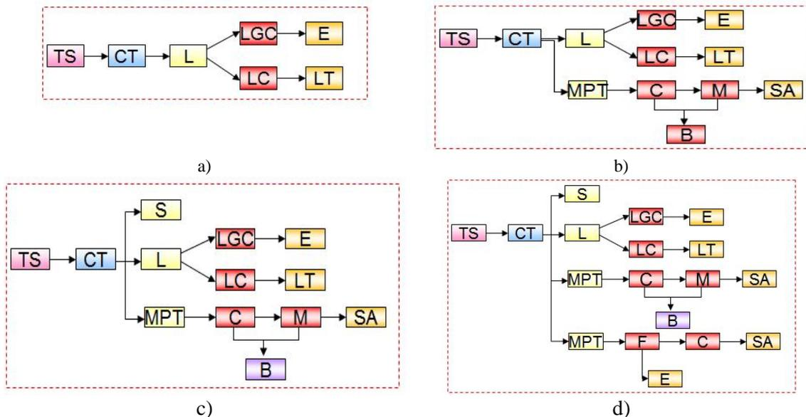
Figure 3. Scenarios proposed for the analysis of MSW management in Iasi, Romania: a) scenario 1, b) scenario 2, c) scenario 3, d) scenario 4, TS – temporary storage; CT - collection and transport; L - landfilling; LGC - landfill gas collection; LC - leachate collection; E - engine; LT -leachate treatment; MT - mechanical treatment; C - composting; M - maturing; SA - soil application; B - bio-filter; S – sorting; F – fermentation.
