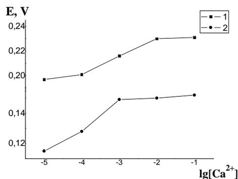
Figure 1. Dependence of the equilibrium potential of the plasticized electrode on concentration of  $\text{Ca}^{2+}$ : 1 – Type 1 electrode (untreated); 2 – Type 2 electrode (pretreated).
