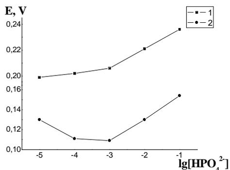
**Figure 2.** Dependence of the equilibrium potential of the electrode on concentration of  $\text{HPO}_4^{2-}$ : 1 – Type 1 electrode (untreated); 2 – Type 2 electrode (pretreated in the  $10^{-3}$  mol/dm<sup>3</sup> solution of  $\text{Ca}(\text{NO}_3)_2$ ).
