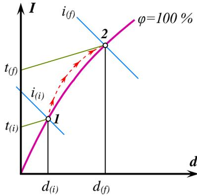
Fig. 3. Diagram I-d representing the air and steam mixing process
