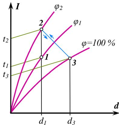
**Fig. 1. Diagram I–d representing the single-stage air heating and humidification mode with the values  $t_3 = t_{\text{rated}}$  and  $\varphi = 100\%$**
