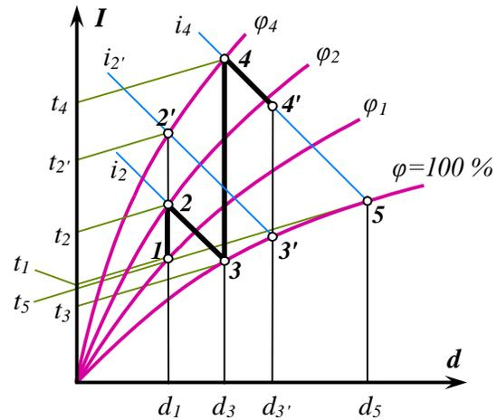
**Fig. 2. Diagram I–d representing the two-stage air preparation process**
