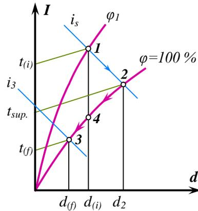
Fig. 4 Scheme for sequencing the operations in Diagram I-d
