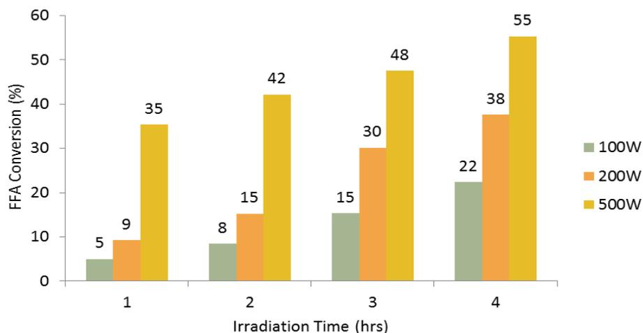
**Fig. 3. Effect of irradiation time and lamp power on photochemical esterification of the waste cooking oil in the absence of a photocatalyst**
