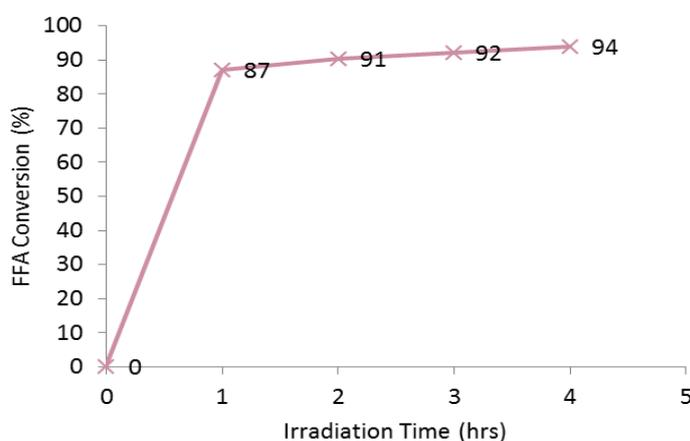
**Fig.4. Effect of irradiation time on photocatalytic esterification of waste cooking oil using ZnO/silica composite and 500 W lamp**
