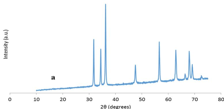
Fig. 1. XRD patterns of the synthesized ZnO/silica composite
