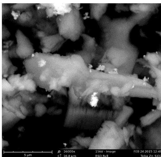
Fig. 2. Scanning electron micrographs of the synthesized ZnO/silica composite
