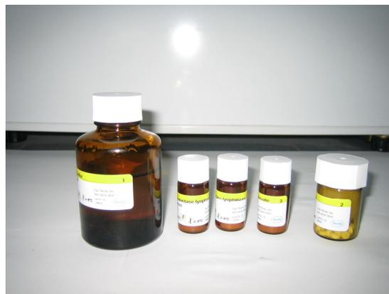
Figure 1. Kit for nitrates determination through enzymatic method
