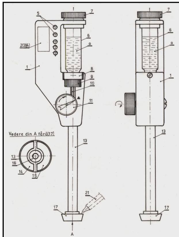
**Fig.3.Exterior front and side of enzyme biosensors, 1-body, 2- electronic unit acquisition, data processing and display, 3-amperometric electronic unit, 4- conductometric electronic unit, 5-keyboard, 6- plastic capsules, o- oxidase solution, 7-bolt, 8-marker, p-drill, f-strip, c-con, 9-nut, 10-silicone hose, 11-cylinder eccentric supported, l-conical seat, 13-rod 14.15 platinum electrodes, 16-con, 17-cup, 21- pipette or manually hoppers.**
