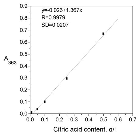
**Figure 3. The calibration curve for citric acid**
