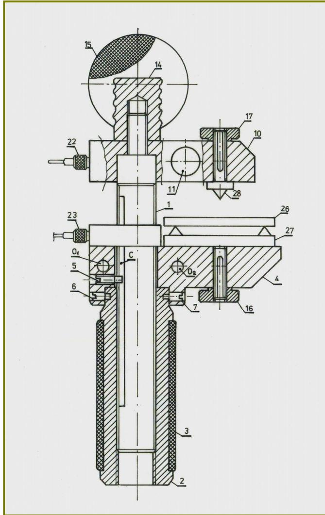
**Figure 1.** Cross-section on side view of the portable device for determining the texture of food and advanced characterization of their behavior to the mechanical testings. 1-screw, 2-nut, 3-liner rubber, 4-lower jaw, 5,6,7,8-screws, 9-displacement sensor, 10-upper jaw, 11-electronic dynamometric cell, 14-nut, 15-spherical rubber body, 16,17-knurled screws, C-guiding channel,  $O_1$ ,  $O_2$ -holes, [11]
