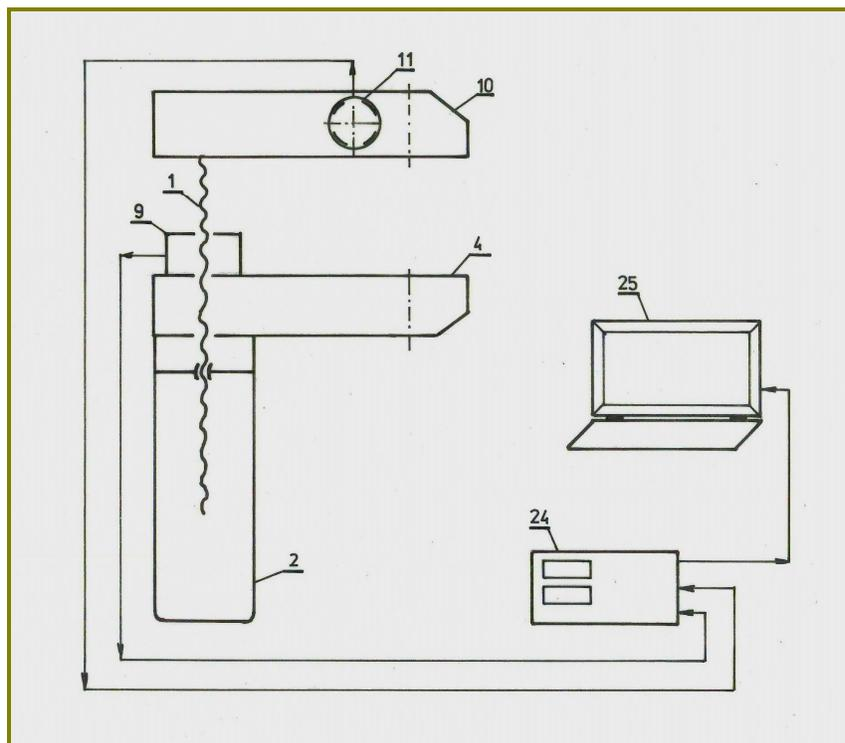
Figure 3. Schematic diagram and kinematic of device for determining food texture and advanced characterization of their mechanical behavior. 1-screw, 2-nut, 4-lower jaw, 9-displacement sensor, 10-upper jaw, 11-electronic dynamometric cell, 24-electronic unit, 25-computing unit, [11]
