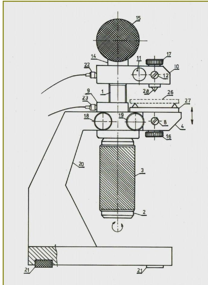
**Figure 2.** Side view of apparatus for determining food texture and advanced characterization of their behavior to mechanical tests and laboratory version with supporting apparatus stand: 1-screw, 2-nut, 3-liner rubber, 4-lower jaw, 8,12-guide screws 9-displacement sensor, 10-upper jaw, 11-electronic dynamometric cell, 14-nut, 15-spherical body rubber, 16,17,18,19- knurled screws, 20-metallic stand, 21-rubber supports, 22,23-electrical connectors, [11]
