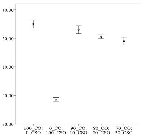
Fig. 2. Variation of Iodine value (IV) in oil samples formulation: CO –corn oil; CSO – coriander seed oil. Error bars show the variations of two determinations in terms of standard deviation.
