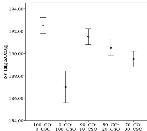
Fig. 3. Variation of Saponification value (SV) in oil samples formulation: CO – corn oil; CSO – coriander seed oil. Error bars show the variations of two determinations in terms of standard deviation.
