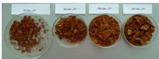
**Figure 7. Comparison of the amount of peeled-off fragments from corrosion layer after 30, 60, 180 and 365 days of exposition of the test samples in water.**
