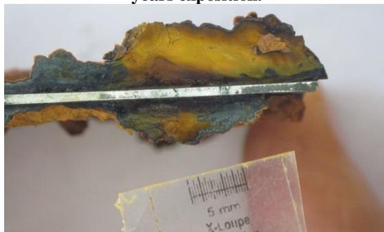
**Figure 6. Photomicroscope's detail of the corrosion layer after two years exposition.**
