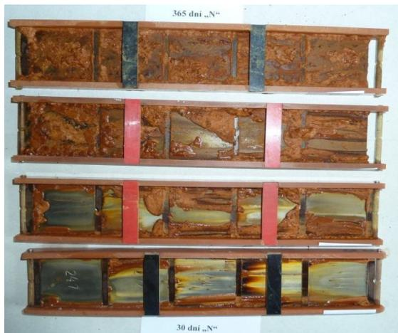
**Figure 4. Development of corrosion layer over time (30, 60, 180, 365 days). Plastic racks with samples are ordered by exposure time, whereas the lowest is the shortest time exposure (30 days).**
