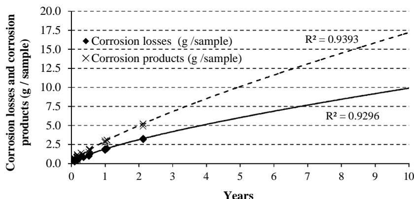
Figure 3. Trend of corrosion losses and corrosion products and their extrapolation
