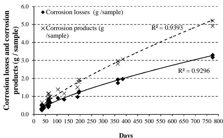
Figure 2. Trend of corrosion losses and corrosion products
