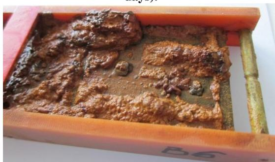
**Figure 5. Detail of the corrosion layer after two years exposition.**
