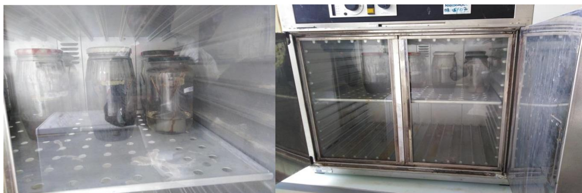
Fig. 1. Experimental set-up for determining cashew nut desorption isotherms
