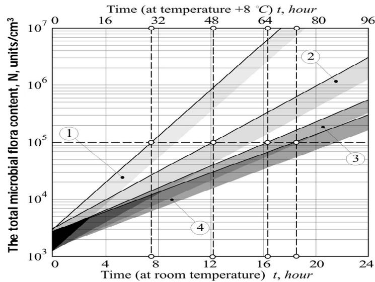
Fig. 5. Development of microflora in milk drinks obtained by sonochemical processing with an amplitude of sound pressure in the reactor of 2.5 bar and acoustic energy: 1 - 0 kJ, 2 - 30 kJ, 3 - 60 kJ, 4 - 90 kJ.
