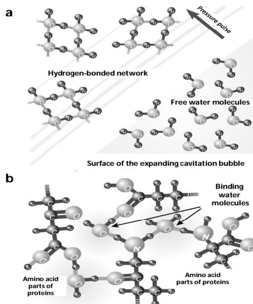
Fig. 2. Schematic representation of hydrogen-bonded network destruction due to cavitation effect of ultrasound (a) and released free water molecules incorporation into proteins (b).
