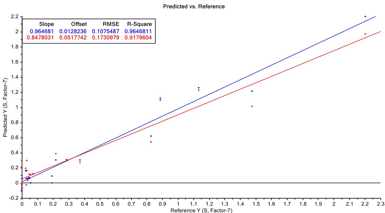
Fig. 2. Reference vs predicted fructose, glucose and sucrose content using FT-IR spectra and PLS-R
