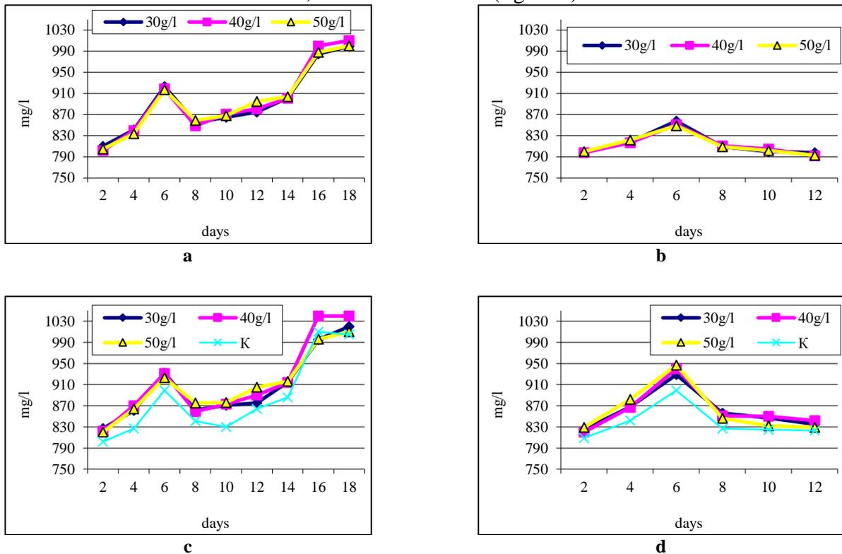
**Figure 4.** The change of total mineralization values of medium using natural form and thermally calcined tuffs: *M. macrocopa* (a) and *S. vetulus* (b) with natural tuffs; *M. macrocopa* (c) and *S. vetulus* (d) with thermally calcined at 150 °C tuffs
