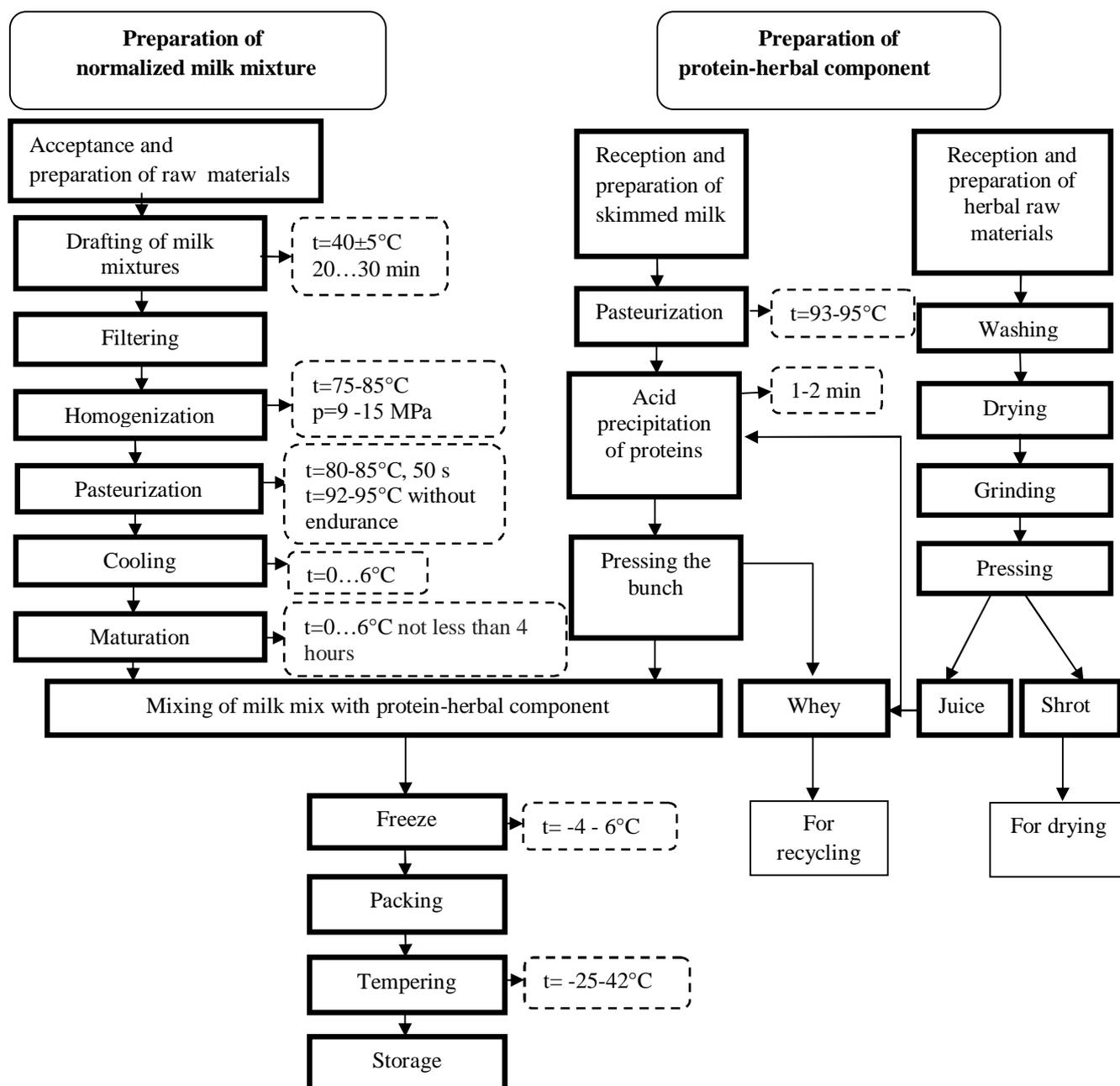
Fig. 2. Parametric scheme of production of frozen dessert with protein-herbal component
