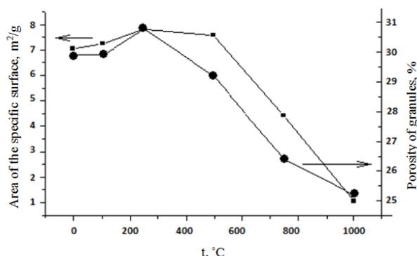
Figure 1. Influence of the modification temperature on the BT's specific surface area and porosity
