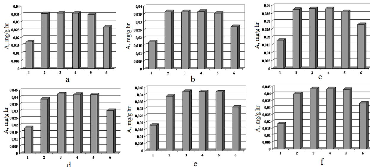
Figure 3. Catalytic activity of the chemically modified tufa samples in the system H<sub>2</sub>O<sub>2</sub> – NaOH – H<sub>2</sub>O C<sub>0</sub>(H<sub>2</sub>O<sub>2</sub>) = 0.05 (a); 0.1 (b); 0.2 (c); 0.4 (d); 0.8 (e); 1.6 (f) M/l: 1 – untreated BT; 2–6 – after modification with HNO<sub>3</sub>, HCl, H<sub>2</sub>SO<sub>4</sub>, H<sub>3</sub>PO<sub>4</sub>, NaOH correspondingly.
