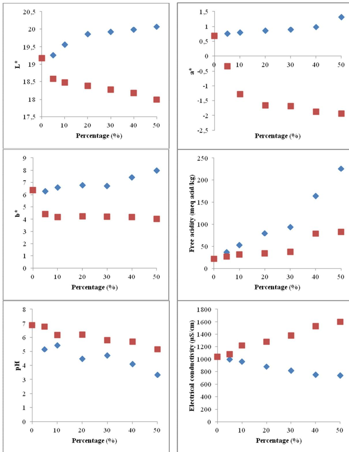
Fig. 1. The evolution of physico-chemical parameters in function of adulteration agent (rhombus –inverted sugar, square - malt wort) and adulteration agent percentage
