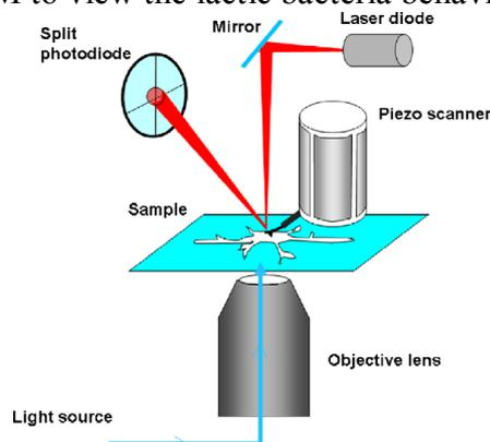
**Fig.4 Scheme of an AFM coupled with an inverted optical microscope [17]**
