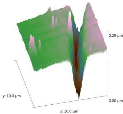
**Fig. 5a The image of a micro channel with 0.29 μm thickness**
