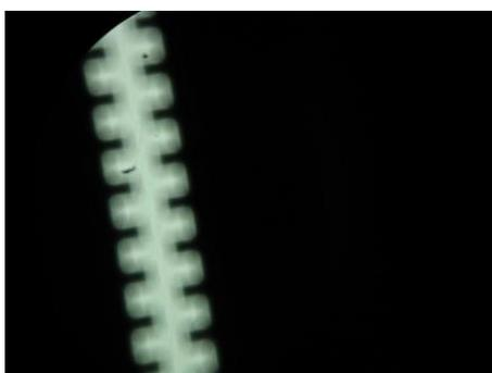
**Fig. 3a Dielectrophoretic chamber with "teeth" electrodes. This image is made at biophysics department UMF Bucharest**
