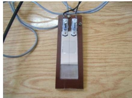
**Fig.6b Dielectrophoretic chamber**
