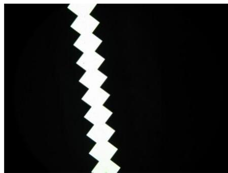
**Fig. 3c Dielectrophoretic chamber with castellated electrodes. This image is made at biophysics department UMF Bucharest**
