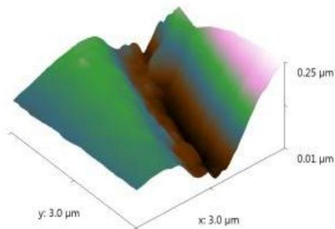
**Fig. 5b The image of a micro channel with 0.25 μm thickness**
