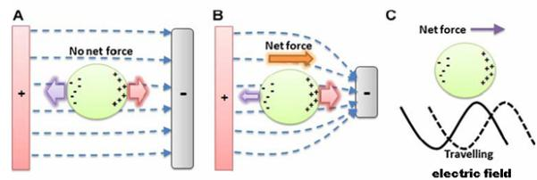
Fig. 2 (a) Uniform electric field resultant force acting on the particle is zero.
