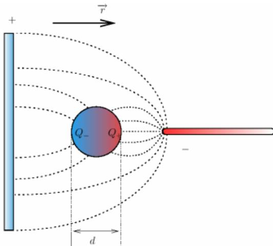
Fig.1 Dipole placed in irregular electric field [16]
