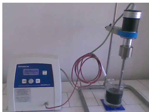
**Fig.2 CNTs suspension ultrasonication using BANDELIN HD3200 as generator**
