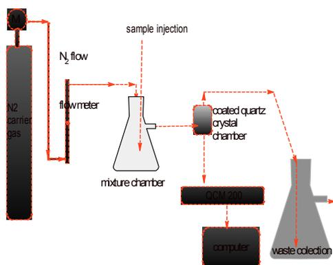
Figure 1. Experimental set-up for the calixarene-coated PQC sensor and amines.
