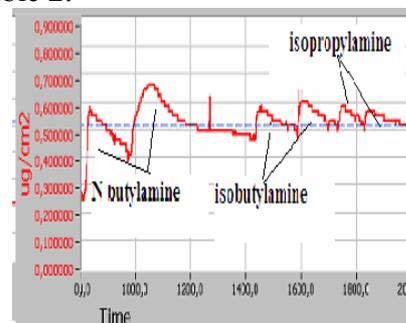
Figure 3. The response characteristics of PQC sensors coated with calyx[6]arene to 40 ppm of 3 organic amines.
