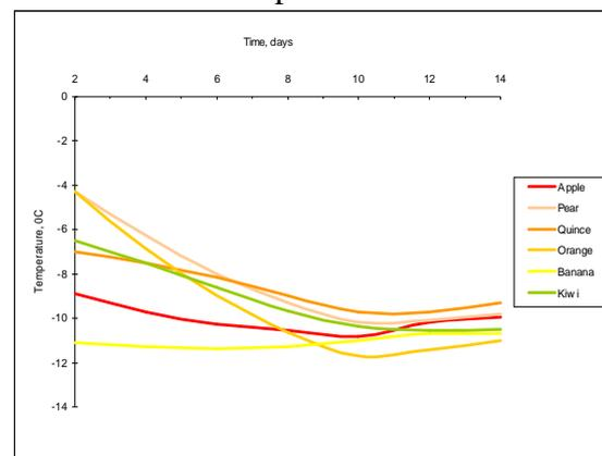
Figure 8. The core temperature variation of freeze packed fruits
