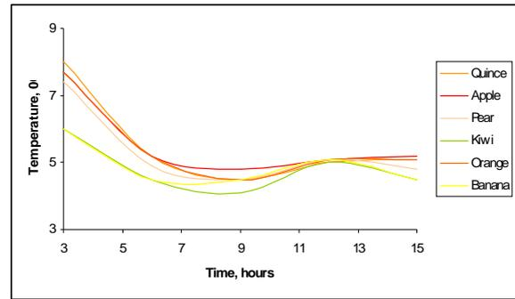
Figure 1. The cooling rate of the bulk fruits at refrigeration
