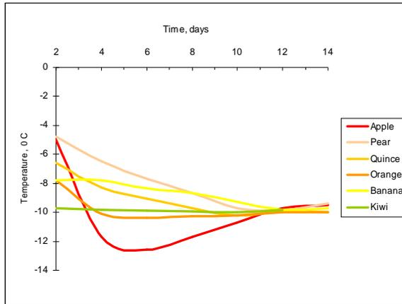
Figure 6 The core temperature variation of freeze bulk fruits
