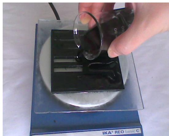
**Fig.2 The dispersion process of CNTs in polyester matrix in a vibrant magnetic field**
