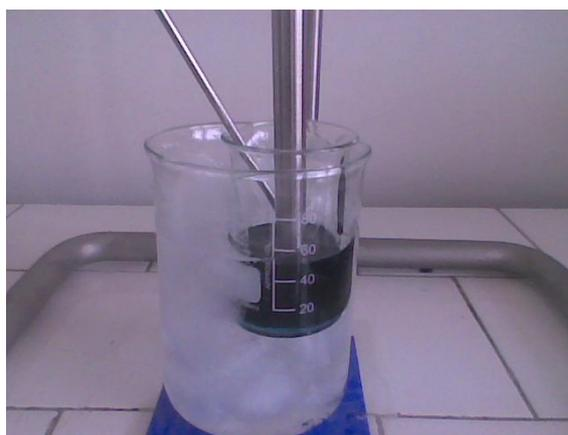
**Fig.1 The dispersion by ultrasonication process in polyester matrix**
