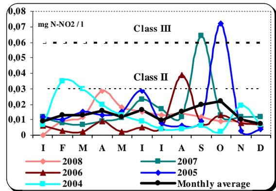
Fig. 11 Evolution of the concentration of N-NO<sub>2</sub> by section Siret - Siret (2004-2008)
