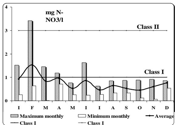
Fig. 12 The average change, monthly minima and maxims on N-NO<sub>3</sub> by section Siret - Siret (2004-2008)
