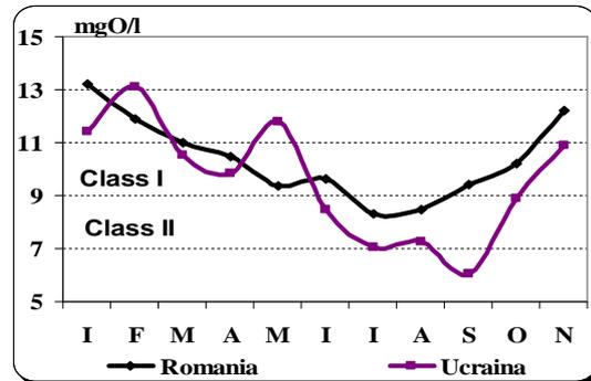
Fig. 5 Comparative evolution of the concentration of dissolved oxygen - section Siret Siret (2008)
