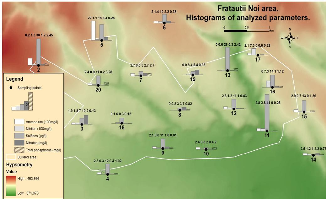
Figure 5. The values of the analyzed parameters and the sampling points in Fratautii Noi
