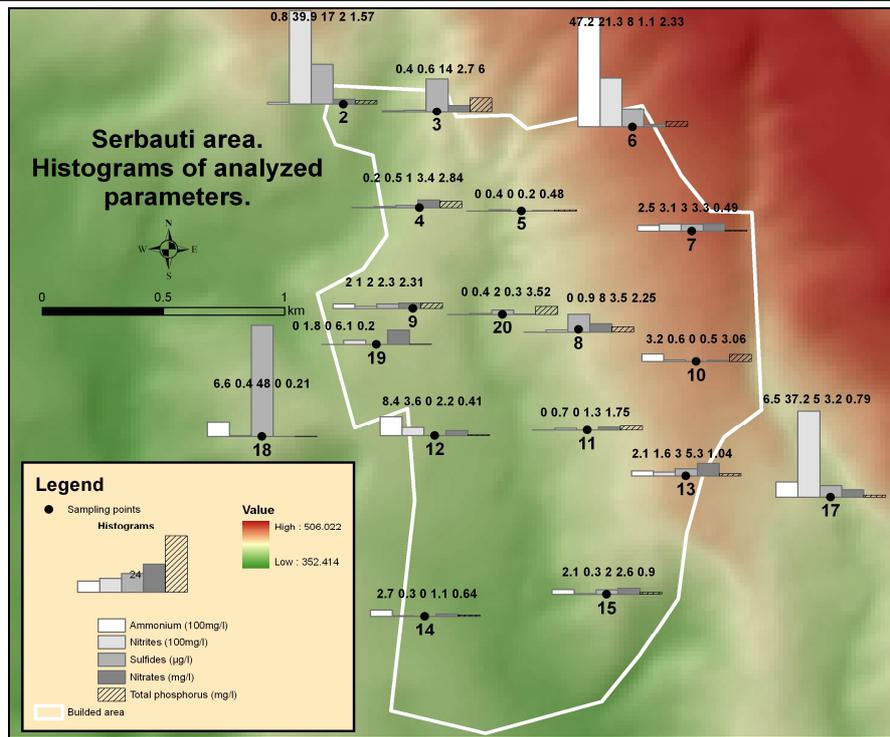
Figure 7. The values of the analyzed parameters and the sampling points in Serbauti
