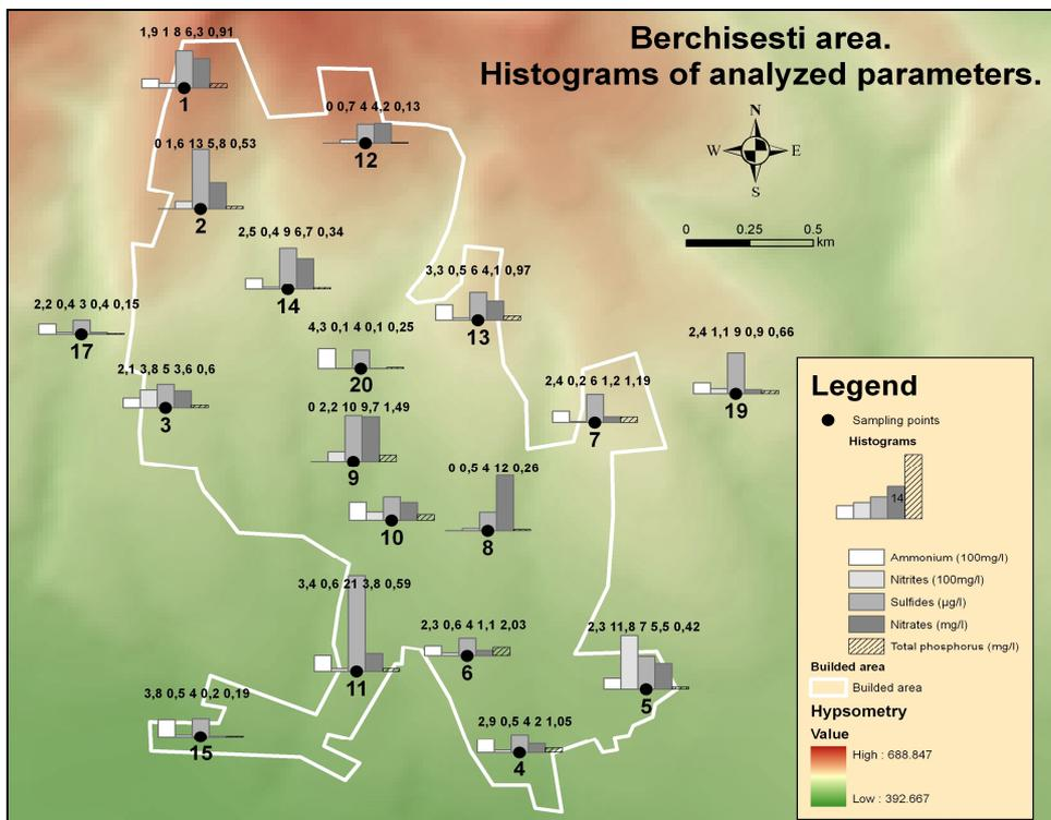
Figure 4. The values of the analyzed parameters and the sampling points in Berchisesti
