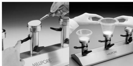
Fig. 1. Work equipment for membrane filtration method
