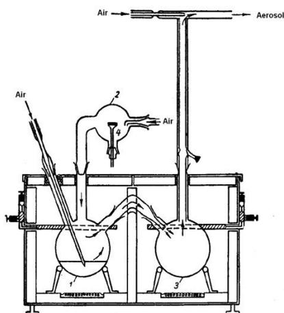
**Figure 1.** The generator scheme by Sinclair and La-Mer (1949) for production of monodispersed particles. Systems for vapor and heterogeneous seeds generation are numbered as (1, 2, 4); vapor superheater has number (3).
