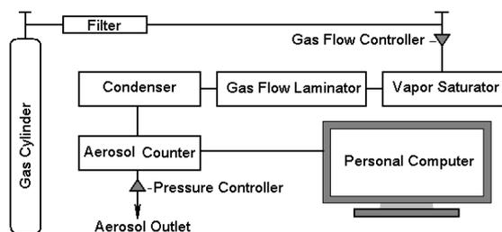
Figure 2. The present day block-scheme of the flow diffusion chamber by Anisimov *et al.* (2001).
