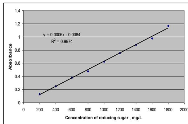
Figure 1. Calibration curve for determination of reducing sugar by DNS method
