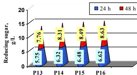
Figure 5. The alkaline-peroxidic pretreatment and the enzymatic hydrolysis at 50°C
