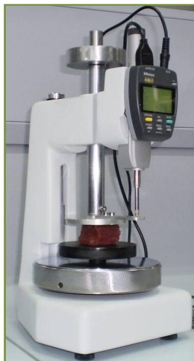
Fig. 1. Device for determining the creep of food products
