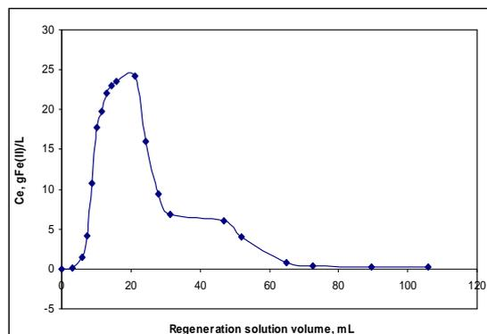
Figure 7. Variation of eluent concentration with solution regeneration volume. 2 g resin dose. flow 0.3ml/minute. HCl 2N.
