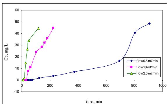
Figure 4. Variation of the effluent concentration depending of operating time.
