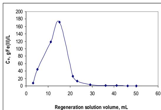
Figure 8. Variation of eluent concentration with solution regeneration volume. 4 g resin dose. flow 0.3ml/minute. HCl 10%.
