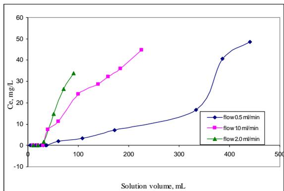
Figure 3. Variation of the effluent concentration depending of volume passed
