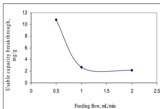
**Figure 2. Variation of usable breakthrough capacity with feeding flow.**
