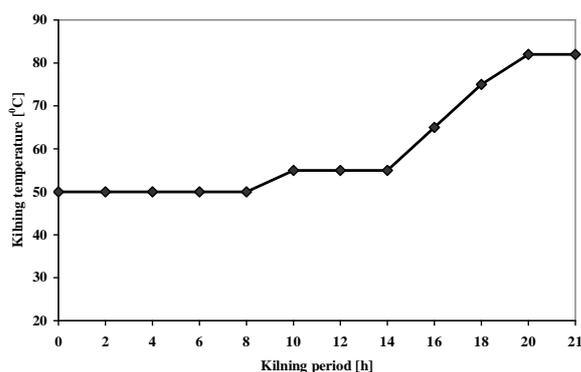
Figure 2. Kilning diagram for all experimental versions
