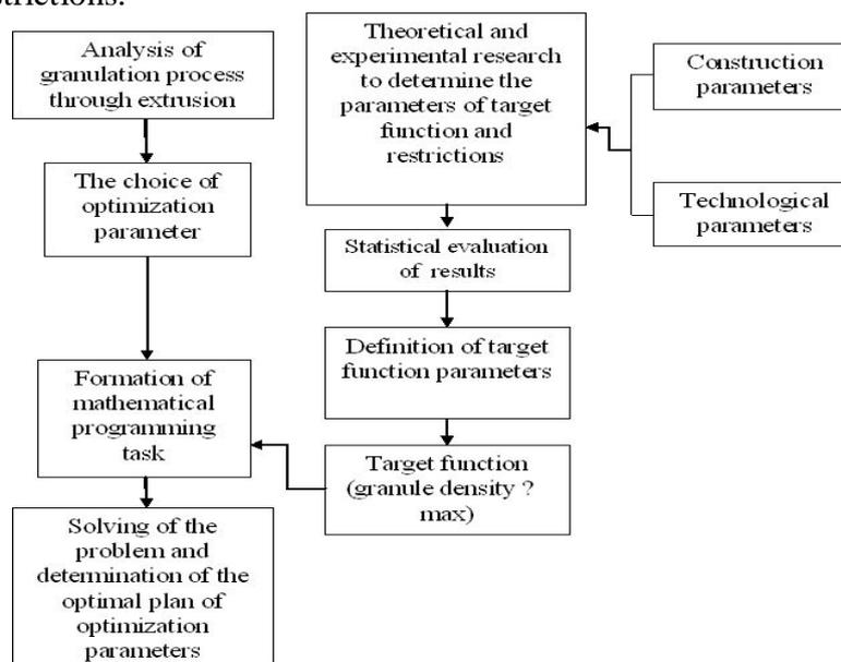
Fig 1. The scheme of determination of optimal constructional and technological parameters of disperse materials granulation through consolidation
