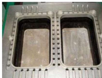
Figure 1. Chamber of the packaging machine with packaging trays
