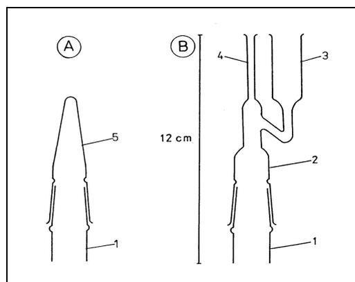
Fig.1 Solvent thin layer separator for microextraction of water
