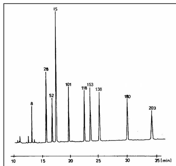
**Fig. 5** Chromatogram of the selected PCB congeners in the concentration of 0.05 µg/l H<sub>2</sub>O.
