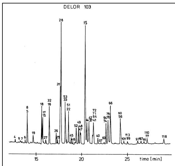
Fig. 2 Chromatogram of the Delor 103 mixture
