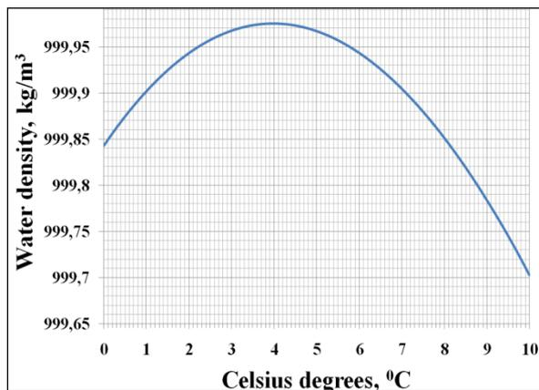
Fig. 1. Correlation of water density from the temperature
