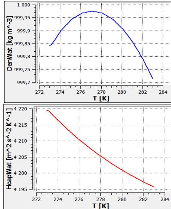
Fig. 5. Water density and heat capacity in the vicinity of inversion point
