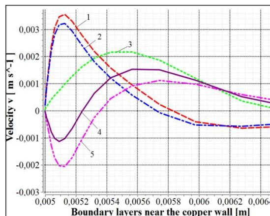
**Fig. 8. Water velocity distribution throughout the high of experimental section in the boundary layer: 1, 2, 3, 4, 5 – velocity throughout the height of experimental section 0.1 m; 0.15 m; 0.06 m; 0.058 m; 0.059 m consequently**
