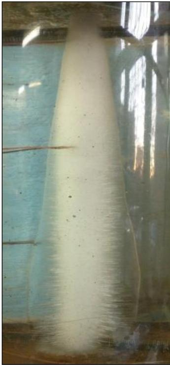
**Fig.10. Ice generation with clear conical shape**
