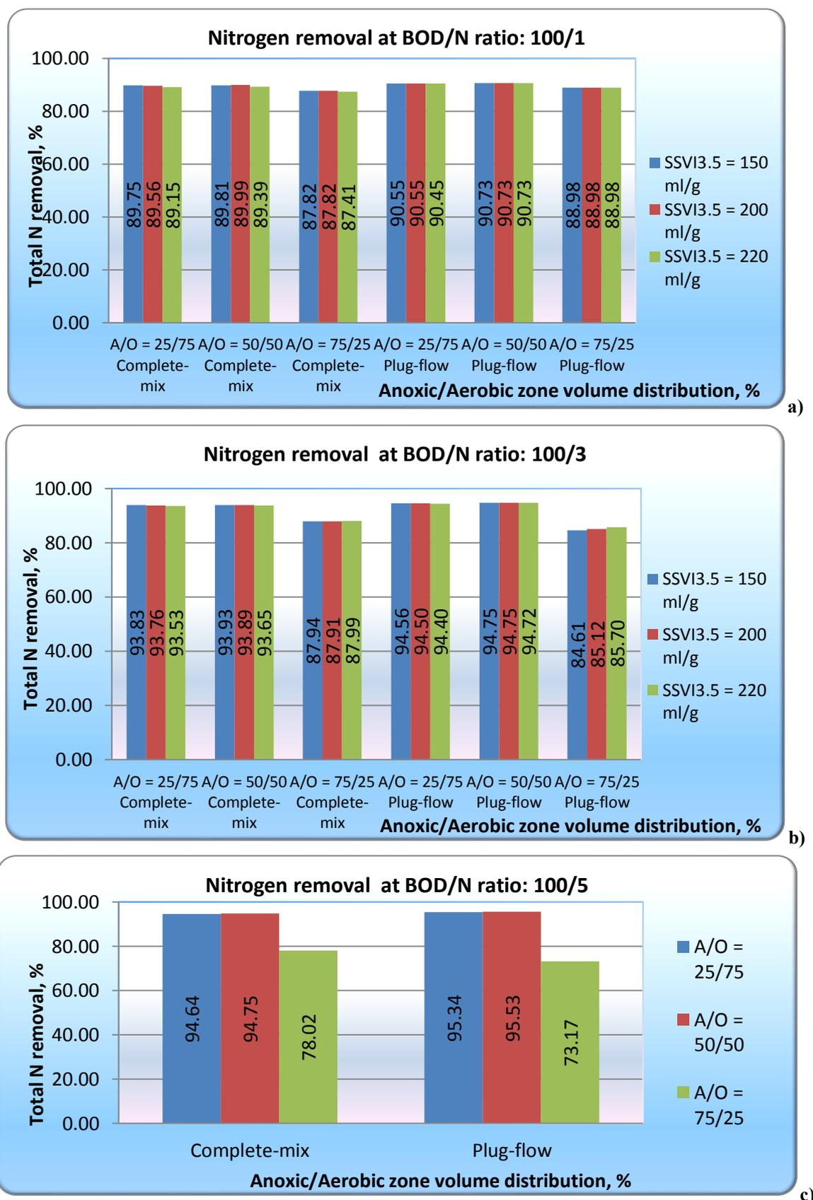
Figure 2. Total nitrogen removal in biological complete-mix and plug-flow unit from wastewater with BOD/N ratio: a) 100/1; b) 100/3; c) 100/5.
