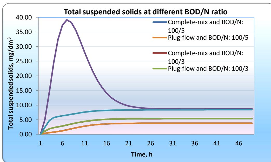
Figure 5. Total suspended solids in the effluent at different reactor system and BOD/N ratio.
