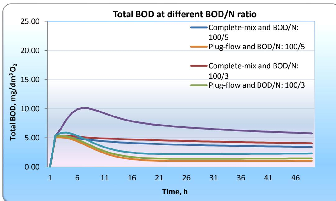
Figure 4. Total BOD in the effluent at different reactor system and BOD/N ratio.
