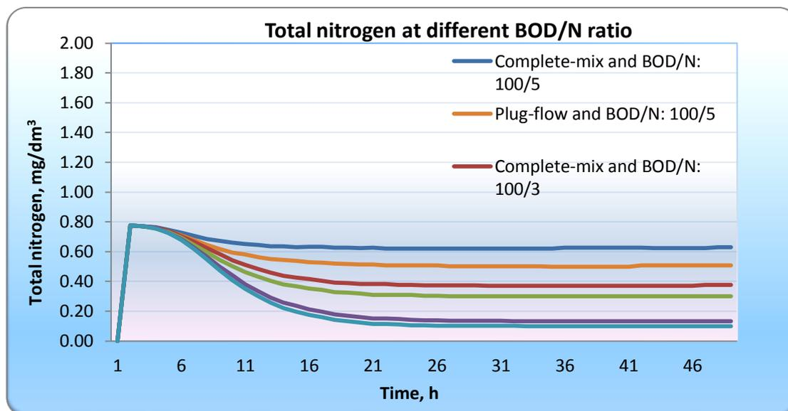
Figure 3. Total nitrogen in the effluent at different reactor system and BOD/N ratio.
