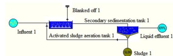
Figure 1. Schematic representation of biological wastewater treatment unit in STOAT<sup>®</sup>.
