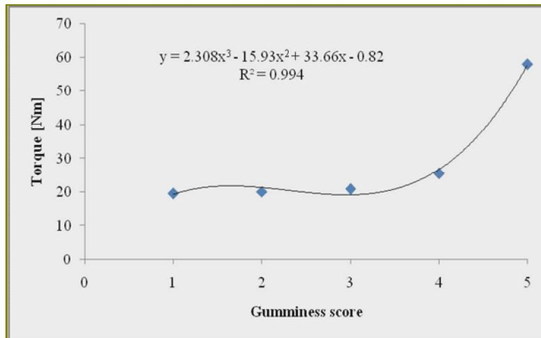
Fig.6. Conversion scale of resistive moment value, measured on the propeller stirrer, in gumminess units as they are defined as the reference standard [1]. All values correspond to the speed of 150 rpm of propeller stirrer
