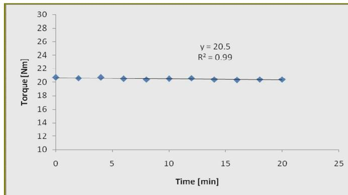
Fig.5. Variation in time of resistive moment of dough with 50% flour and 150 rpm of propeller stirrer.
