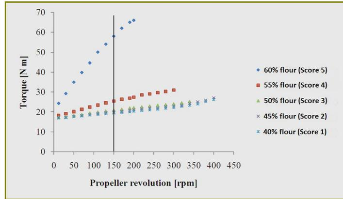
Fig.4. Graphic cumulative representation of resistive moment evolution depending on the speed at different concentrations of flour-water according to [1] and tab.2. highlighting resistive moment at 150 rpm
