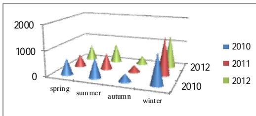
Fig.11. Values of total nitrogen content of waste water before treatment
