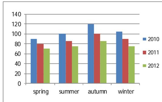
Fig. 16. Values of oil and fats content from waste water after treatment
