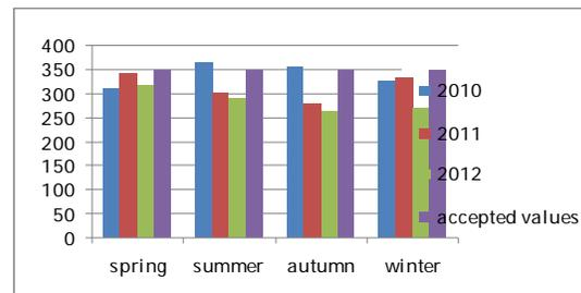
**Fig.6 Values of suspended solids content in waste water after treatment**
