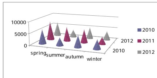
**Fig.5. Values of suspended solids content in waste water before treatment**
