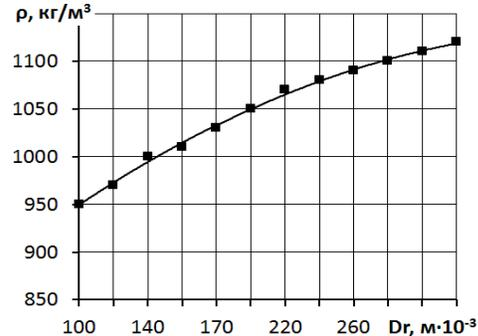
Figure 7.d. Density dependence of  $\rho$  pellets on  $D_r$  roller diameter
