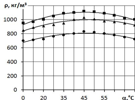
Figure 7.c. Density dependence of  $\rho$  pellets on  $\alpha$  hole matrix angle
