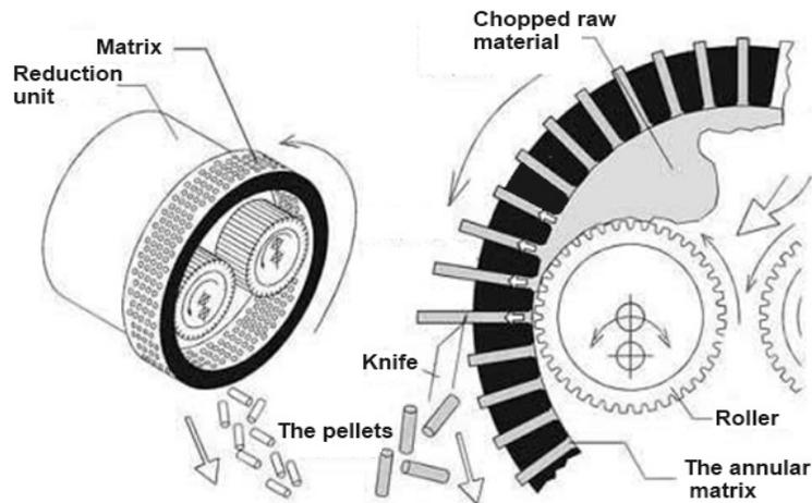
Figure 2. Granulator unit with annular matrix
