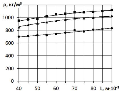
Figure 7.b. Density dependence of  $\rho$  pellets on  $L$  hole matrix length
