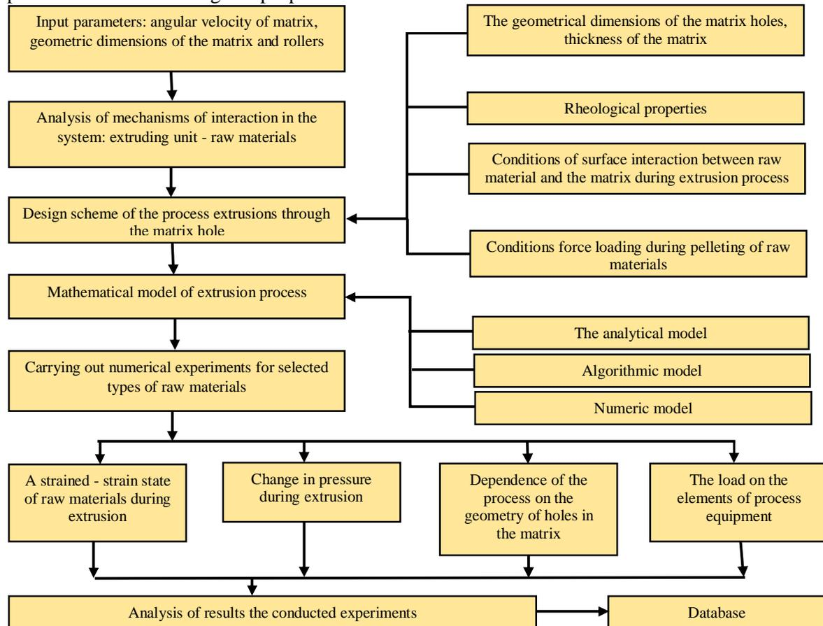
Figure 1. Information technology scheme of designing equipment for extrusion compacting.
