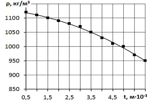
Figure 7.e. Density dependence of  $\rho$  pellets on  $t$  air gap size between roller and matrix
