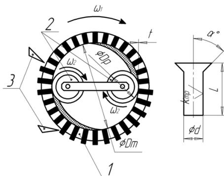
Figure 3. Scheme of work of the granulator unit
