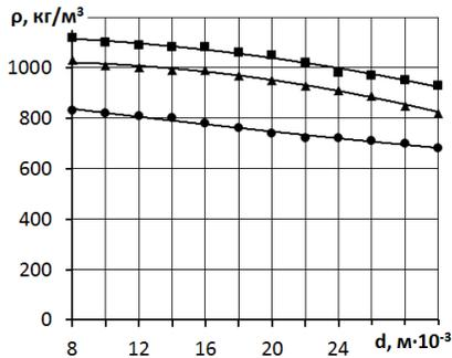
Figure 7.a. Density dependence of  $\rho$  pellets on  $d$  hole diameter
