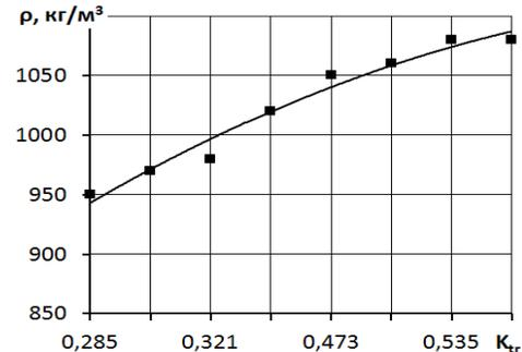
Figure 7.f. Density dependence of  $\rho$  pellets on friction coefficient between DM and matrix
