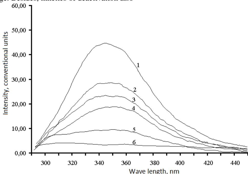
**Figure 1.** The intrinsic fluorescence spectra of BSA after bubbling of the ozone-oxygen mixture (ozone content 7,0 mg/l) during various periods of time. 1 – control experiment (no ozone mixture bubbled); 2 – 0,5; 3 – 1; 4 – 2,5; 5 – 4; 6 – 6 min. Exciting radiation wavelength – 280 nm.
