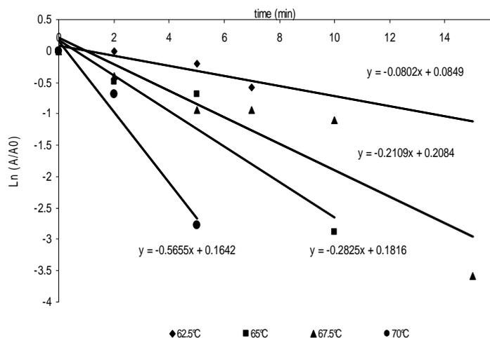
**Figure 5. Thermal inactivation kinetics of the LPO in whey**
