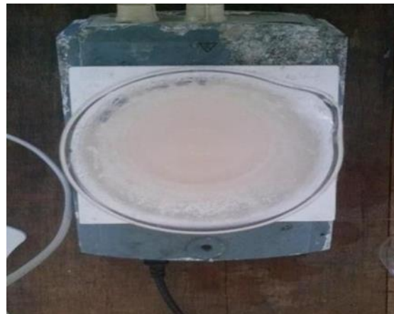
Fig. 3 Bio-plastic prepared by film casting
