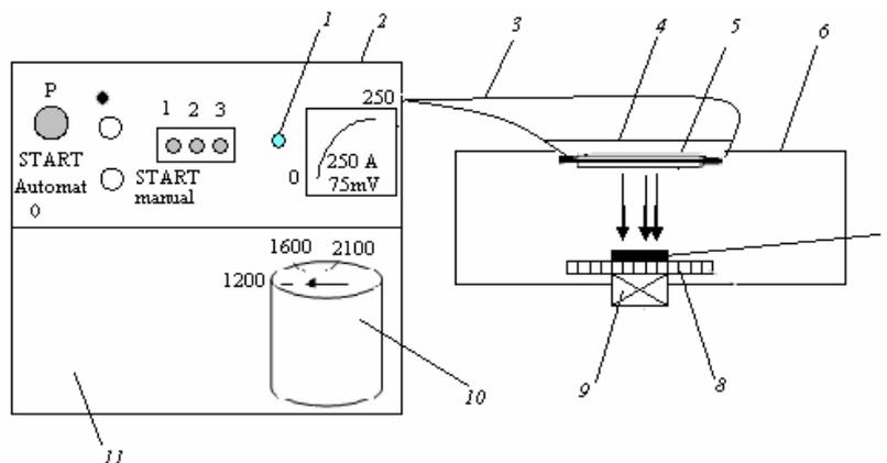
**Figure 1. Pulsed light installation 1 – led; 2 - pulse generator; 3 – control cable; 4– lid; 5- IFP-800 flash lamp; 6 – treatment space; 7 – glass pieces spreaded with mould spores; 8 – plate of wire sieve; 9 – support system; 10– energy autotransformer; 11 – system with five capacitors.**
