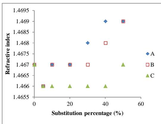
**Fig. 1. Refractive index evolution: A- virgin olive oil substituted with sunflower oil, B- virgin olive oil substituted with corn oil and C – virgin olive oil substituted with groundnut oil**
